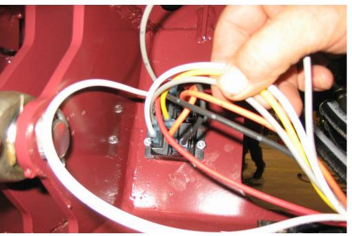
THE <u>BLACK #5 WIRE W/ JUMPER WIRE</u> is now jumpered to the <u>bottom/right terminal on the BOTTOM</u>
