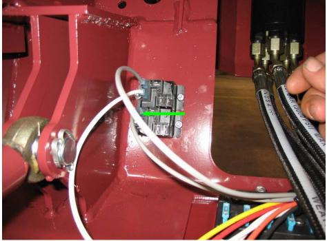
**GREY #9 WIRE** connects to the bottom relay – to the terminal shown just below the **WHITE #3 WIRE**.
