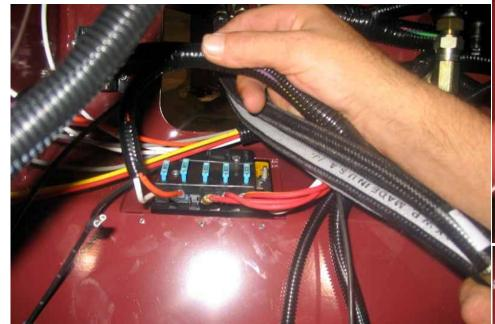
Connect the <u>RED/YELLOW #20 WIRE</u> to the <u>bottom</u> right terminal on the fuse box. The <u>RED/GREEN #21</u> WIRE connects next to the <u>RED/YELLOW #20 WIRE</u>.
